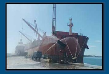
A Water Curtain has been placed with a water recycling system around the operational area and this system has been implemented by spending a minimum cost and we have been able to mitigate the dust emission using this method.
